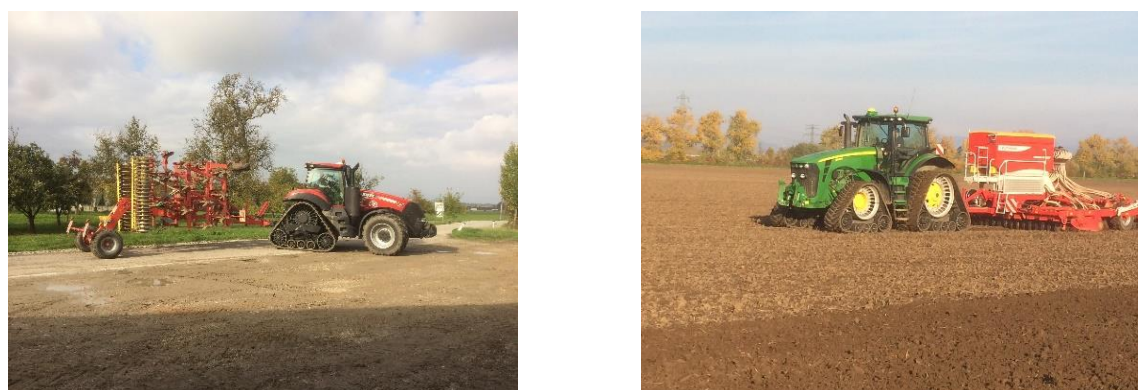
Fig. 10. Half-tracked (left) and fully-tracked (right) AWD-tractor with rubber tracks
