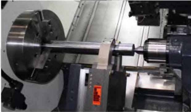
Fig. 1. Clamping of workpiece
